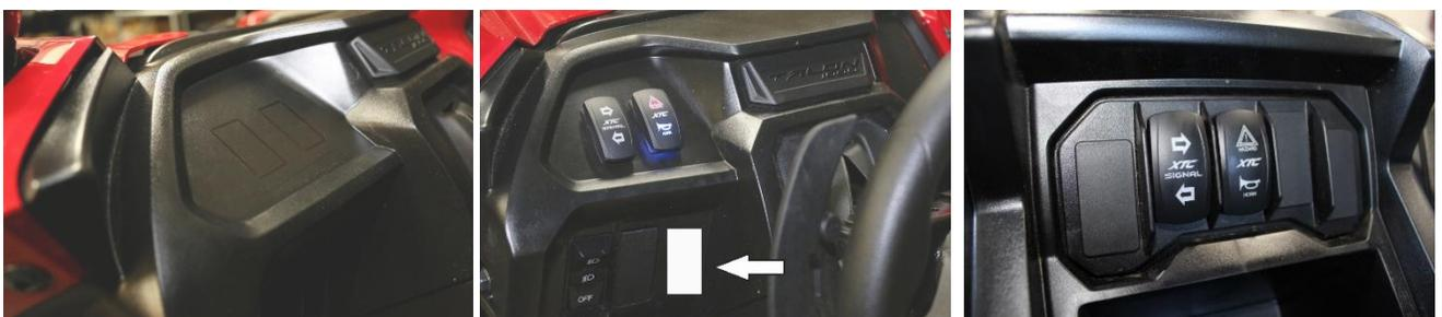
**Dielectric Grease** - Just like the OEM uses on their switches, we recommend using Dielectric Grease on all switch terminals, this keeps the water out, thereby reducing corrosion and helps increase reliability! Open the grease and put on the switch terminals and the connector terminals on the Horn switch.
