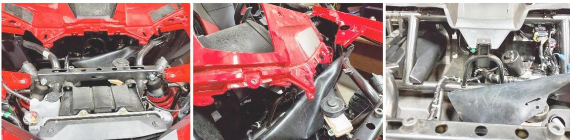
Remove Center Console Plastics and Rear Box Cover to run rear harness.
