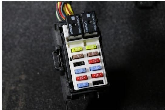
12. Plug the fuse adapter into F28 as shown below.
