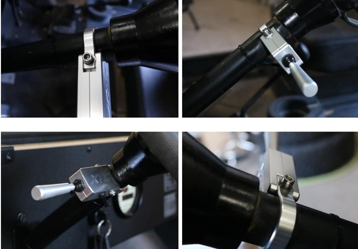
7. **Run the wire harness –** down the column and secure with the included cable ties.
