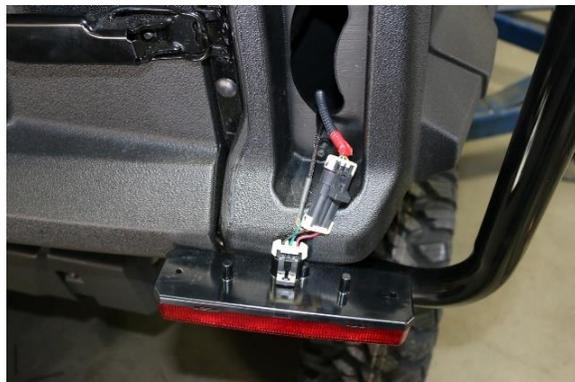
6. Run the wire down to the trailer hitch.
