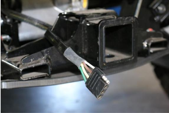
7. Verify operation of adapter and rear taillights and secure all installed cables with supplied cable ties.
