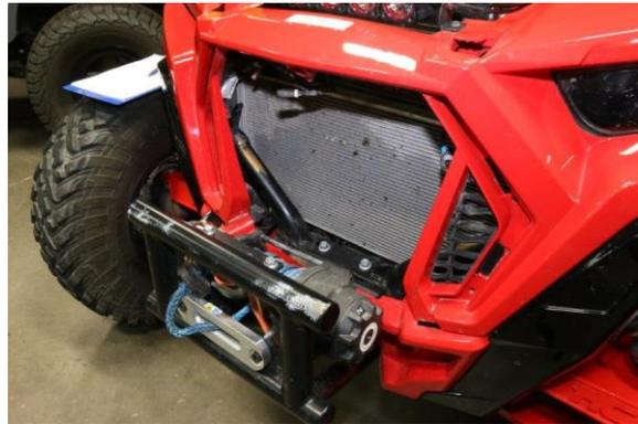
2. Run the harness – Set the harness on the cross member, run one of the 2 Pin Connectors to the right opening and one to the left opening.
