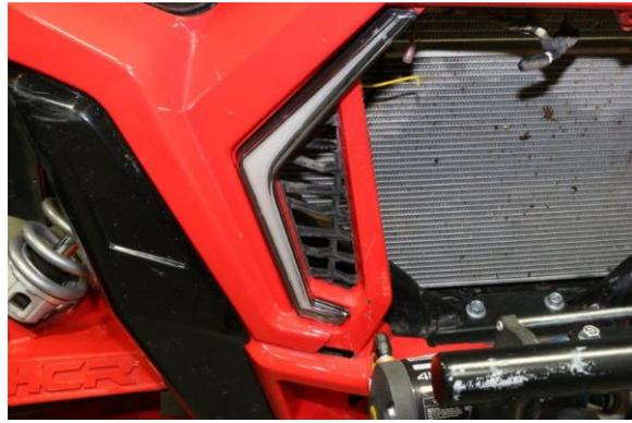
4. Attach the Red Wire to the left Accessory Post on the Factory Busbar. Attach the Black Wire to the Ground Post.
